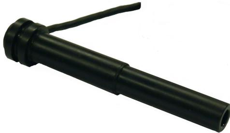
An on-plug coil for use with high current transistorised (inductive) ignition (TSI) as available in all our ECU's. Design and manufacture is in-house, so we can make the coil to suit your specific application. The information given here is for a typical coil. Many of the parameters can be tailored to a particular installation.
